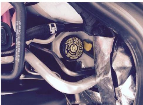
2. Open the bonnet, identify where the brake fluid reservoir is and tell me how you would check that you have a safe level of hydraulic brake fluid.
