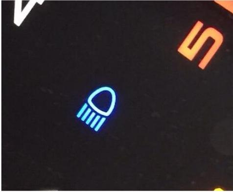
18. Show me how you switch your headlight from dipped to main beam and explain how you would know the main beam is on whilst inside the car.
